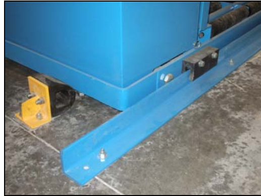
Vehicle Guidance via Angle Track / Guide Block with Cushioned Floor Stop (Positive Engagement & Precise Alignment with Batteries)
