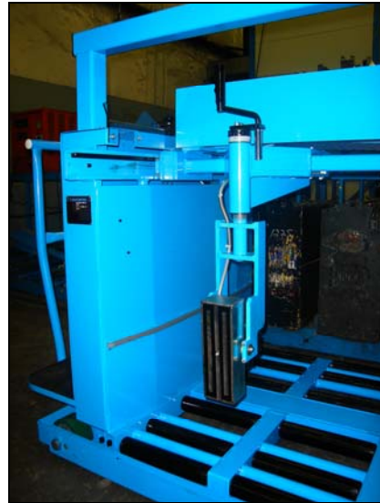
Enclosed Operators Platform & Free Flowing Roller Bed (10K Option & Extended Yoke Shown)
