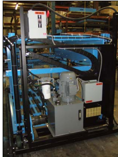
Power End of Unit with Cover Removed
